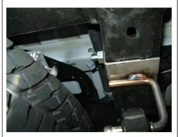
**Step 4.** At this point you will need to install the provided Hanger Bracket Assembly onto the D/S frame rail to allow for the installation of the dual system. Install the bracket to the frame rail with the supplied 1/2" fasteners and the backing plate for the backside of the rail. Fasten the Supplied Rubber Insulator to the hanger once mounted.
