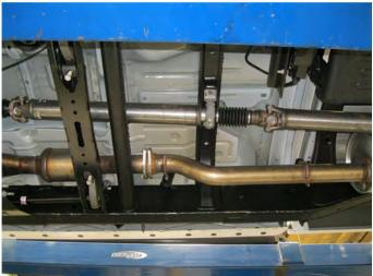
**Step 1.** To remove the OEM exhaust system you will need to cut the pipe behind the muffler before it goes over the axle. Disengage the welded hangers from the rubber insulators and remove the tailpipe. Next remove the fasteners from the two bolt flange behind the catalytic converter. Do not damage or discard the fasteners or rubber insulators, as they will be re-used to mount the new system. Disengage the remainder of the hangers and remove the system.
