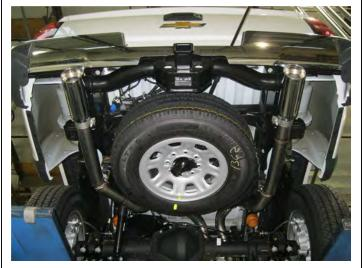
**Step 5.** Finish by installing the Tail Pipe Assemblies to the over axle Extension Pipe Assemblies and the Tips to the Tail Pipe Assemblies using the supplied 3.00" clamps and fitting the welded hangers into rubber insulators. Use the two < 3.00x7.00" Extension Pipes between the Tail Pipe Assemblies and the Tips if your truck has a Long Bed configuration.
