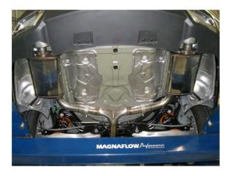
**Step 4.** Finish by installing the Muffler Assemblies to the Y-Pipe Assembly using the supplied 2.50" clamps, and fitting the welded hangers into the rubber insulators.
