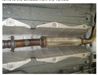
**Step 2.** To begin, fasten the Resonator Assembly inlet to the catalytic converter using the provided fasteners and gasket (Leave all clamps and fasteners loose for final adjustment of the complete system.)
