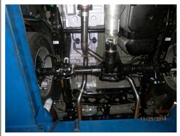
**Step 5.** Continue the installation by loosely attaching the Over Axle Assemblies to the Muffler using a supplied 2.50" clamp and inserting the hanger into the rubber insulator.
