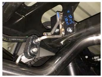
**Step 6.** Loosely install the Tail Pipe Assemblies in a similar fashion using the supplied 2.50" clamps. Attach the supplied hanger bracket as shown using the supplied hardware. The mounting holes in the bracket will align with pre-existing holes in the vehicles sub frame. Attach the Hanger Bracket to the welded hanger on the drivers side Tail Pipe Assembly using the supplied Hanger Rubber.
