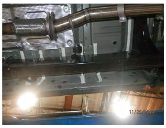
**Step 3.** Begin installing of the new system by attaching the Inlet Pipe Assembly to the flange re-using the OEM fasteners and inserting the hanger into the rubber insulator.
