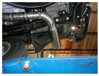
**Step 4.** Complete the installation by attaching the Tail Pipe Assembly to the Muffler using a supplied 3.00" clamp and inserting the hanger into the rubber insulator.
