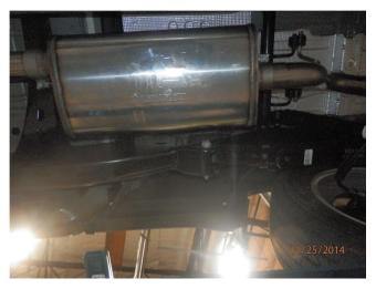
**Step 3.** If your vehicle has a Crew Cab with a Standard Bed configuration you will need to include the supplied 14.50" Extension Pipe between the Inlet Pipe Assembly and the Muffler. For Crew Cab/Short Bed and Extended Cab/Standard Bed the Extension Pipe is omitted. Next loosely attach the Muffler to the Inlet Pipe Assembly or the Extension Pipe using a supplied 3.00" clamps.
