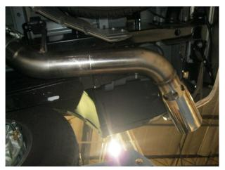
**Step 3.** Finish by loosely installing the Tail Pipe Assembly to the Inlet Pipe Assembly using a supplied 5.00" clamp and fitting the welded hanger into the rubber insulator.
