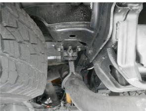
**Step 1.** To remove the OEM system, begin by unclamping the Extension Pipe from the junction behind the DPF. You can then disengage the welded hangers from the rubber insulators and remove the system. Do not damage or discard the rubber insulator it will be reused to mount the new system.
