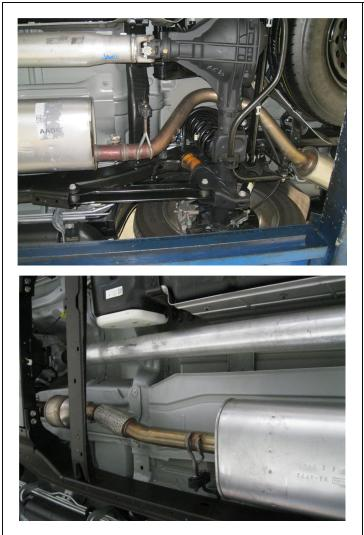
**Step 1.** To remove the OEM exhaust system, you will first need to cut the pipe behind the muffler before it goes over the axle. You can then disengage the welded hangers from the rubber insulators and remove the tailpipe. Unfasten the muffler inlet from the catalytic converter at the clamp junction. Do not damage or discard the OEM fasteners or rubber insulators, as they will be reused to mount the new system. Disengage the muffler hangers and remove it from the vehicle.
