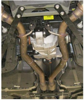
**Step 1.** Begin by removing the two front crossmembers and the two rear chassis stiffeners by the muffler inlets. This will allow access to the exhaust system.
