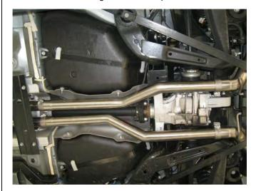
**Step 4.** Next, attach the Driver and Passenger Side Extension Pipes (as shown) to the Resonator Assembly using the supplied 2.50" clamps.
