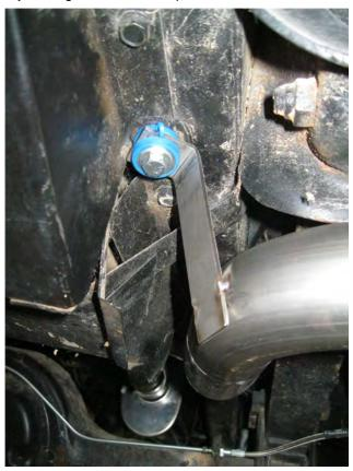
**Step 4.** Install Tailpipe Assemblies using supplied 2.50" clamps. Fit hangers onto installed hangers using the supplied black rubber insulators. Fit hanger brackets to existing threaded holes in the frame rails using the supplied blue grommets and fasteners.
