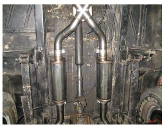
**Step 2.** Next install the mufflers as shown (be aware of orientation) using the supplied 2.50" clamps.
