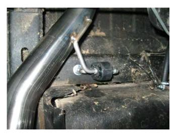
**Step 3.** Before installing the Tail Pipe Assemblies you will need to install the supplied threaded hangers into holes in the frame rails behind the rear differential using two supplied nuts and washers to adjust height and lock into place.
