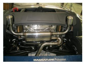
**Step 5.** Next use the supplied 2.50" clamps to attach the Muffler Assembly to the Mid Pipe and the Tail Pipe Assemblies to the Muffler. Fit hangers into rubber insulators.
