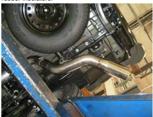
**Step 4.** Finish by installing the Tail Pipe Assembly to the over axle Resonator assembly using the supplied 4.00" clamp, fitting the welded hanger into rubber insulator.
