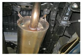
**Step 2.** Disengage hangers from rubber insulators and remove the OEM exhaust.
