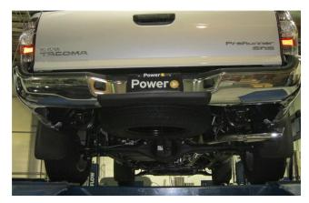
**Step 5.** Once a final position has been chosen for the new exhaust system, evenly tighten all clamps from front to rear using the torque specifications on page one of the instructions. Inspect all fasteners after 25-50 miles of operation and re-tighten if necessary.
