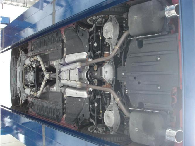
**Step 2.** Install the new system by loosely attaching the new X-Pipe Assembly to the catalytic converter using the OEM hardware and by locating the welded hanger to the rubber isolator. Leave all clamps and fasteners loose for final adjustment of complete system.
