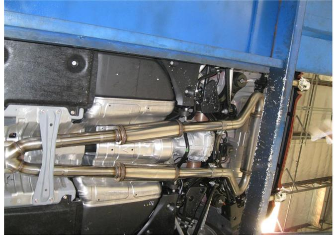
**Step 4.** Loosely secure the Muffler Assembly and both Tip Assemblies in a similar fashion and reattach the cross brace.
