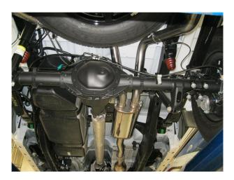
**Step 4.** Working front to rear install the remaining pieces of the MAGNAFLOW system, inserting hangers into rubber insulators and loosley intstalling suppled clamps. Adjustable tips are supplied to fit a variety of aftermarket bumpers and rollpans, once a position is decided for the tips it is recommended to have them welded into place.
