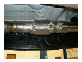
**Step 3.** Install the new Inlet Pipe Assembly at the ball flare using the OEM clamp. Leave all clamps and fasteners loose for final adjustment of the complete system.
