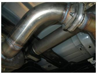
**Step 3.** You are now ready to install your new MAGNAFLOW exhaust system. Begin by bolting the inlet flange of the Muffler Assembly to the Y-Pipe assembly using the OEM hardware. Engage both welded hangers to the rubber isolators.
