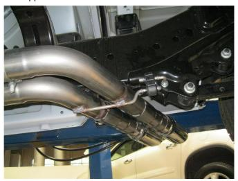
**Step 5.** Next, install the Tail Pipe Assembly by slipping the inlets over the Muffler Assembly outlet pipes. Loosely secure with the supplied clamps. Locate the supplied rubber isolator to the previously mounted hanger and the welded hanger on the assembly.
