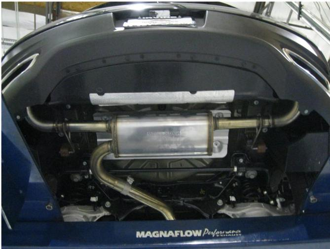
**Step 5.** Next install the Muffler Tail Pipe Assembly by attaching it to the Connecting Pipe with the supplied clamp and engaging all welded hangers to the rubber insulators. Locate both tail pipes to the OEM exhaust tip shrouds.
