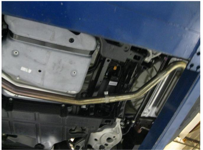
**Step 4.** Loosely install the Mid Pipe to the Resonator Assembly and Connecting Pipe using the supplied 2.50" clamps.
