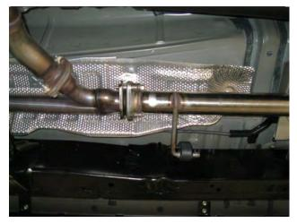
**Step 3.** You are now ready to install your new MAGNAFLOW system. Attach the the Inlet Pipe Assembly to the OEM Y-Pipe outlet using the existing hardware. Engage the welded hanber to the OEM rubber insulator. Leave all clamps and hardware loose for final adjustment of the complete system.
