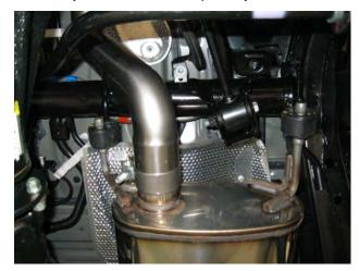
**Step 4.** Slip the inlet of the Muffler Assembly over the outlet of the Inlet Pipe Assembly and loosely secure using the supplied 2.50" clamp and 15mm socket. Engage all welded hangers to the OEM rubber insulators. Install the Mid Pipe and the Tail Pipe Assembly using a similar procedure.
