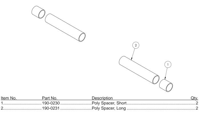
Attach poly spacers to the pivot bar to keep ramps from shifting during transport and loading. These polycarbonate spacers are included in the MAD-RAMPS Snowmobile Kit and are required to make the quick clamps on your center ramp work
