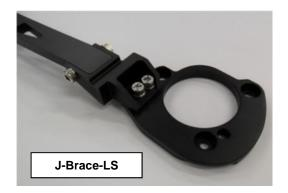
5) Slide the end brackets onto the J Bar. These are designed as a tight fit. Using the two long bolts and corresponding nuts, attach the cross bar to the brackets as shown in the image. Note that with the brackets in the correct position, the bar will be sitting more towards the front of the car. The bolts can only go from the front to the back. The back hole is threaded. Do not tighten.
