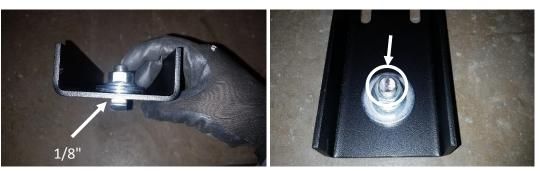
Install the 5/8" clipped head carriage bolt through the upper mounting plate, then install the (2) - 3/4" washers on the carriage bolt along with the 5/8" flange nut. Screw nut down until there is a 1/8" gap between the carriage bolt head and bottom of the upper mounting plate. Align the clipped sides with the bent sides of the bracket and draw a line indicating the direction on the carriage bolt head.
