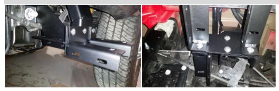
Insert a 3/8" carriage bolt through the step mounting bracket, step support bracket and second step mounting bracket. Hand tighten a 3/8" flange nut on the bolt.
