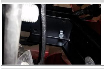
Attach the angle support bracket to the upper mounting bracket by inserting a 1/2" hex bolt through the angle support bracket hole and upper mounting bracket slot then hand tighten a 1/2" flange nut on the bolt. Repeat for remaining 3 holes.
