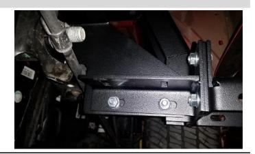
Insert 3/8" hex bolts through the step mounting bracket and lower mounting bracket. Hand tighten a 3/8" flange nut on the bolt.
