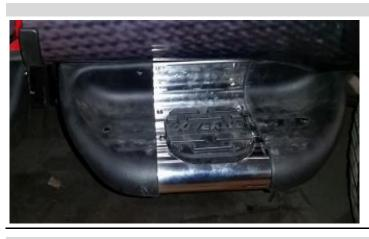
Set the step plate in position on the step mounting brackets. Insert (4) #10-24 carriage bolts through the neoprene washers, step plate and step mounting brackets. Hand tighten a #10 flange nut on each bolt.
