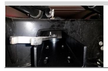
Loosen the flange nut enough to allow the carriage bolt to turn. Rotate carriage bolt 90 degrees then tighten with 15/16" wrench. The black line drawn on the bolt should be used as a visual and a mirror may be needed to see the bolt. The bracket end should be parallel with the side of the truck box.
