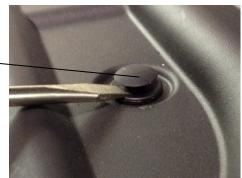
3. UNSCREW THE FOUR SCREWS ON THE TOP OF THE GRILLE, SECURING THE GRILLE TO THE VEHICLE.
