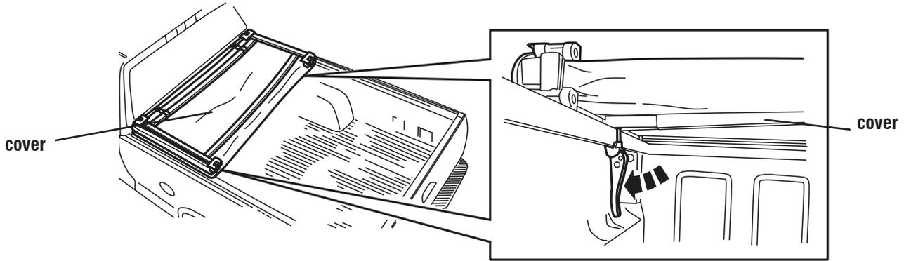
NOTE: Clamp handle must rotate completely down to the stop to be locked. If something interferes with the handle (bed liner, bed extender or cargo, etc.) it must be modified or removed.
