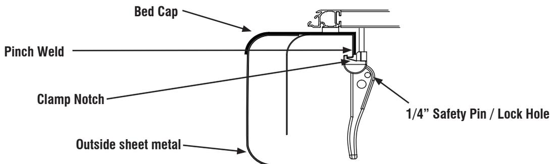
If traveling with the Tonneau in the folded position it is recommended to use a safety pin or lock in the front clamps.
