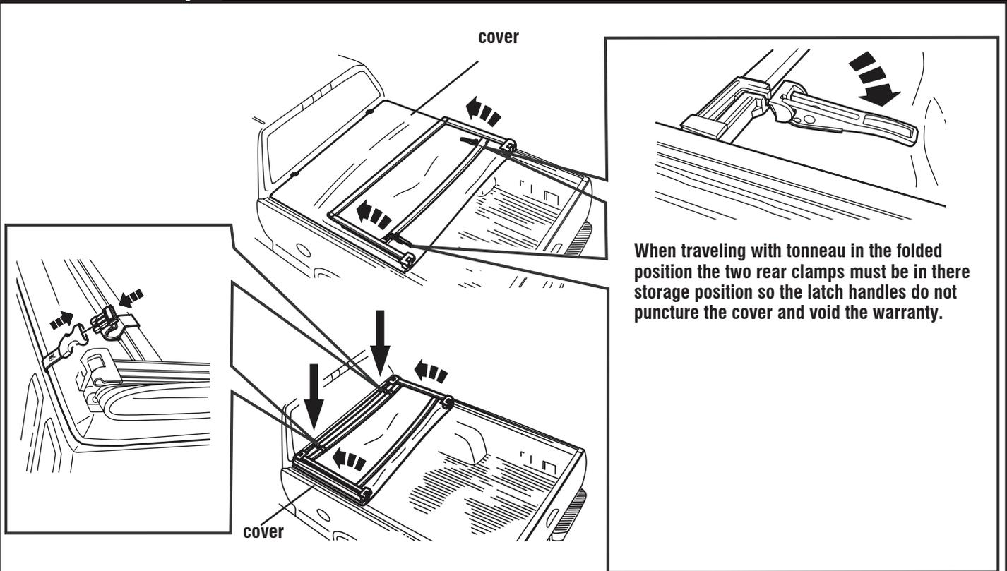
The retaining straps must be buckled when vehicle is in motion if Tonneau is in the folded position.
