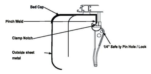
If traveling with the Tonneau in the folded position it is recommended to use a safety pin or lock in the front clamps.
