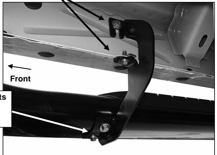
(Fig 9) Passenger side front Bracket installation
