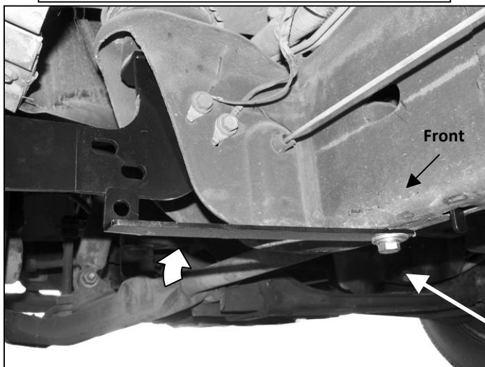
(Fig 5) 25-3500 Model Front Support Bracket Installation Pictured
