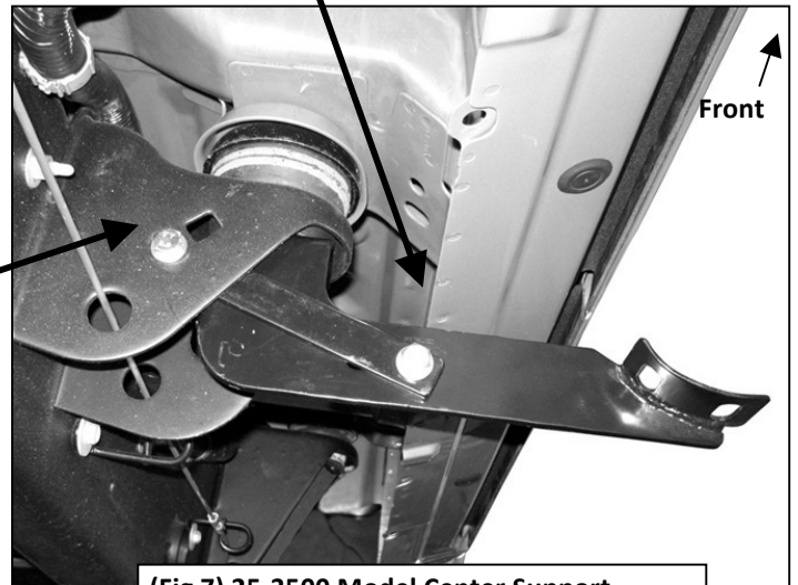
(Fig 7) 25-3500 Model Center Support Bracket Installation Pictured
