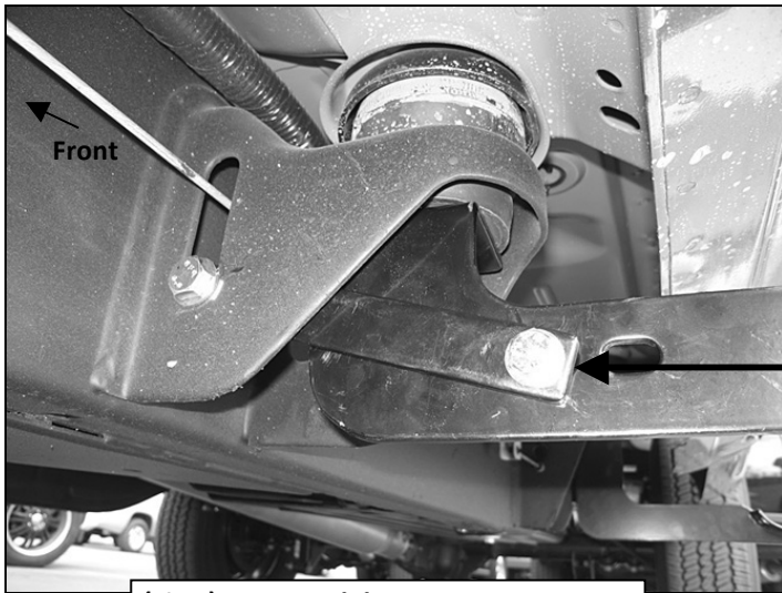
(Fig 6) 1500 Model Center Support Bracket Installation Pictured
