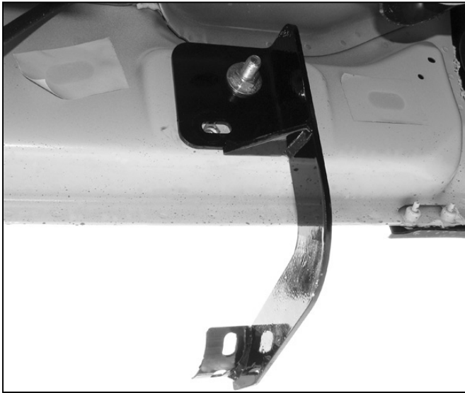
(Fig 3A) Driver/Left front Mounting Bracket
