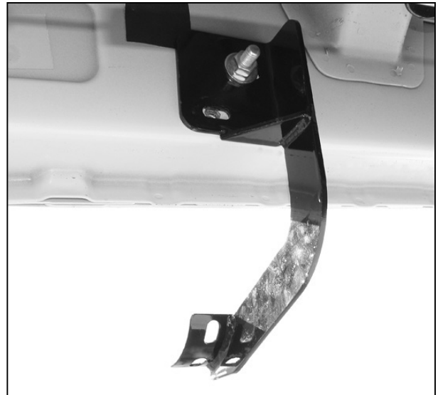
(Fig 3B) Driver/Left center Mounting Bracket
