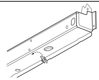
At the front set of diagonal holes, insert bracket from Step 1 into the large hole and into the inner rocker panel. If sound deadening foam is present, press foam to the side providing clearance for bracket. Move the bracket back and forth to make sure it is sitting flat.
