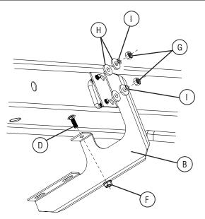
Position bracket over the installed U-bolts, being careful to prevent the U-bolt from slipping into the rocker panel. Slide the bolt of bracket into the upper notch of bracket. (Make sure that the bolt is fully engaged in the slot.) Install remaining fastener and finger tighten nut.
