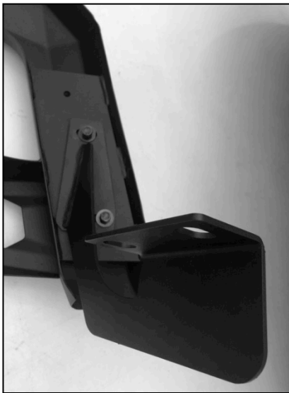
(Fig 7) Attach Bull Bar to Mounting Bracket using M8 Bolt Assembly. (For illustration purposes, shown off vehicle)
