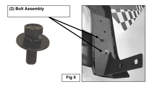
**7.** Center the Bull Bar on the vehicle, level and adjust as desired and tighten all hardware at this time. Check front bumper alignment and readjust as necessary as mentioned in **Step 3**.
