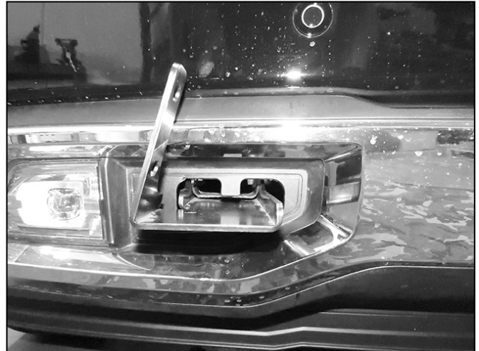
(Fig 11) Passenger/right side Bracket installed
