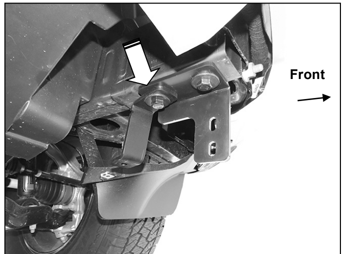
(Fig 7) Driver/left Frame Bracket installed with optional Skid Plate Bracket (arrow)
