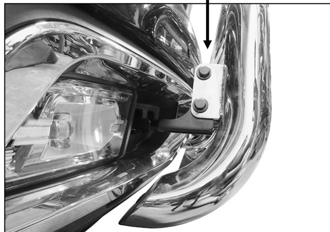
(Fig 13) Passenger/right side complete installation
