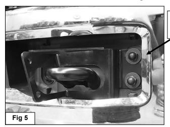
Reuse factory bumper bolts to attach Bracket and Spacer to Bumper
