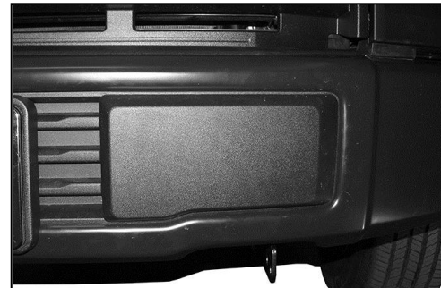
(Fig 5) Remove bumper pads to access splash guard hardware if necessary. 2015 F150 pictured
