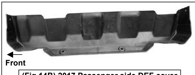
(Fig 14B) 2017 Passenger side DEF cover
