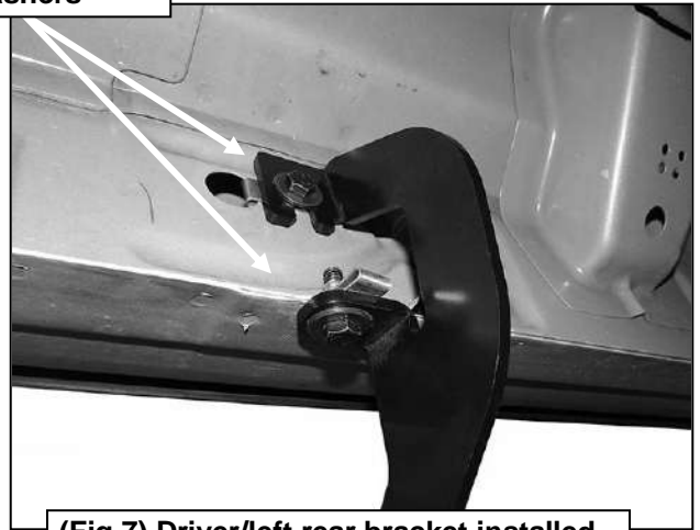
(Fig 7) Driver/left rear bracket installed
