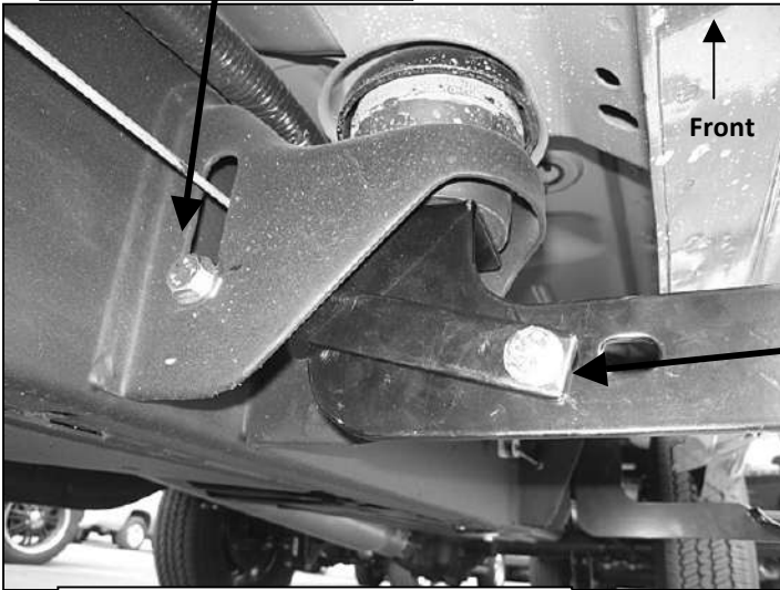
(Fig 6) 1500 Model Center Support Bracket Installation Pictured
