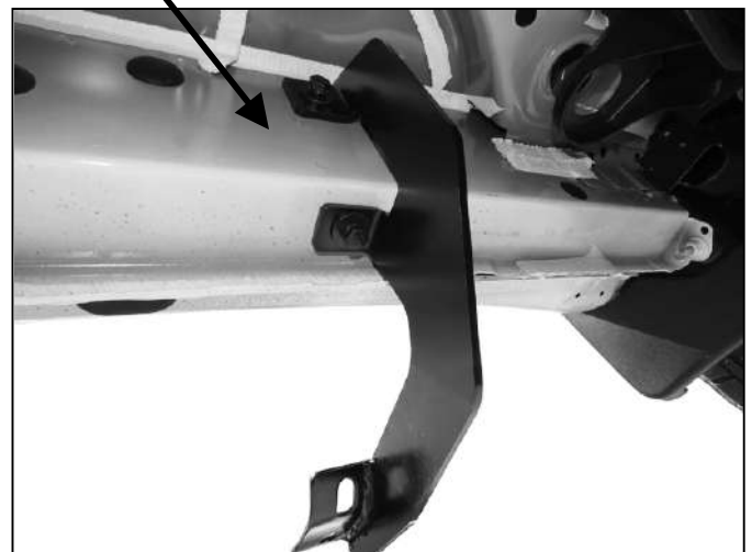
(Fig 4) Driver/left front Bracket installed
