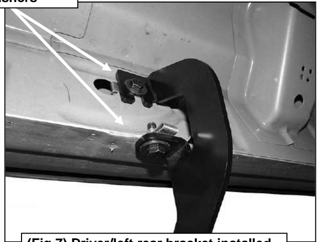
(Fig 7) Driver/left rear bracket installed
