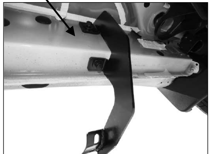
(Fig 4) Driver/left front Bracket installed
