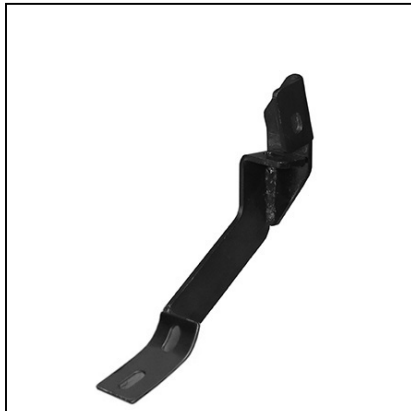
(Fig 15) Passenger/right Front Lower Bracket (all models)
