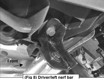
(Fig 8) Driver/left nerf bar attached to Front Bracket
