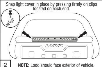
**NOTE:** It may be necessary to use a screwdriver to pry the clips on each end slightly wider to achieve optimal fit.
