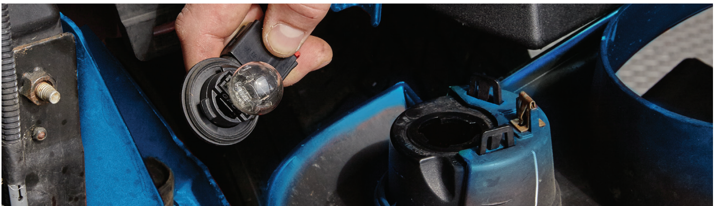
The parking light assembly has already been removed from its location in the grille
