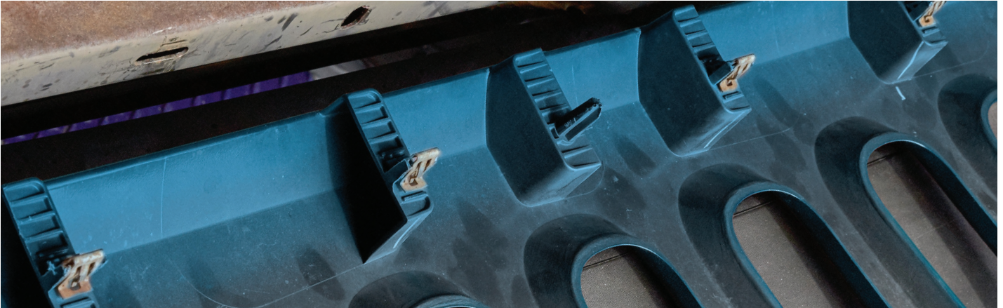
The bottom clips are disengaged by pulling at the bottom of the grille
