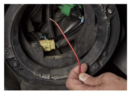
CAUTION! Some Jeeps have TWO 12v accessory sockets, one hot with the key on, and one hot all the time. Select the one which is "on" only with the ignition on. If you select the one which is always hot, the DRL lights will never turn off, and you will drain the battery.
