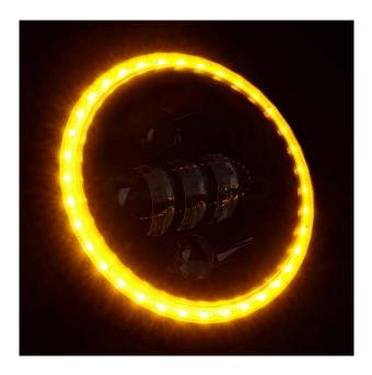
The procedure below results in each halo ring blinking AMBER with its respective turn signal. Should you desire different functionality, you would alter the connections as necessary.
