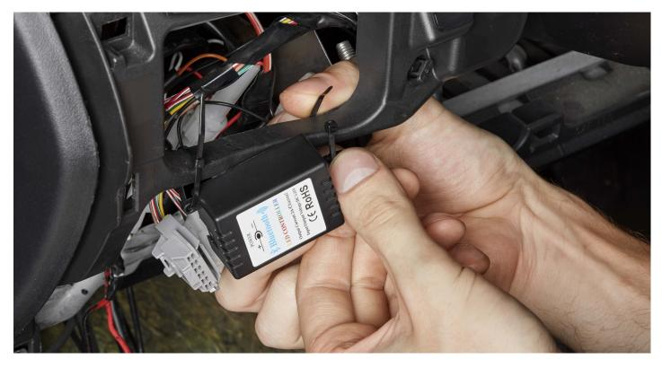
**STEP 9.** Plug the RGB wires into the controller.
