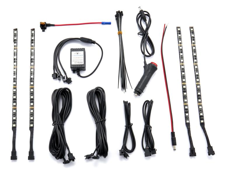
**STEP 1.** Remove all components from box, make sure all parts are present. Using a QR reader scan the QR code included in the controller box and install the application on your smartphone. Plug controller into cigarette lighter and connect all lights, confirm operation of all lights and functions before beginning installation.
