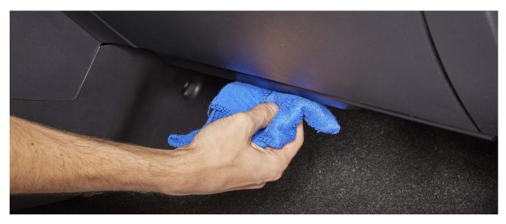
**STEP 4.** Peel the red strip off the adhesive on one side of the strip. Stick the end of the strip onto the mounting surface, peel the remaining red strip off while adhering the light to the mounting location. Repeat this step for the other three lights.
