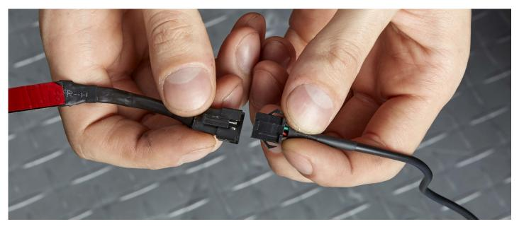
**STEP 6.** Secure all loose and hanging wires with provided cable ties. Move the seats in all positions to make sure the seat movement does not interfere with any of the wires or lights.
