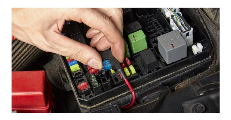
**STEP 2.** Using a butt connector, connect the wire from the add-a-fuse to the end of the power cord pigtail from the Bluetooth controller.
