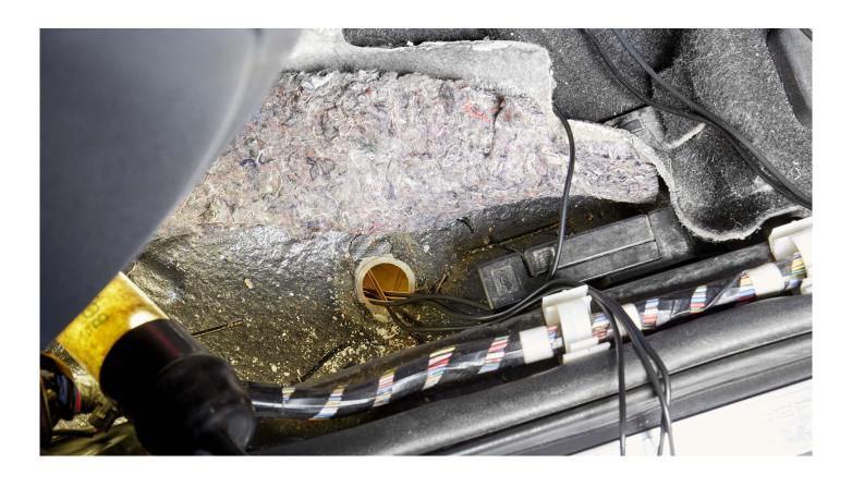
**STEP 6.** Secure all loose and hanging wires with provided cable ties. Make sure the wires are not close to any moving or hot components.
