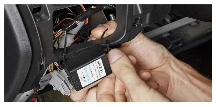
**STEP 9.** Plug the RGB wires into the controller.
