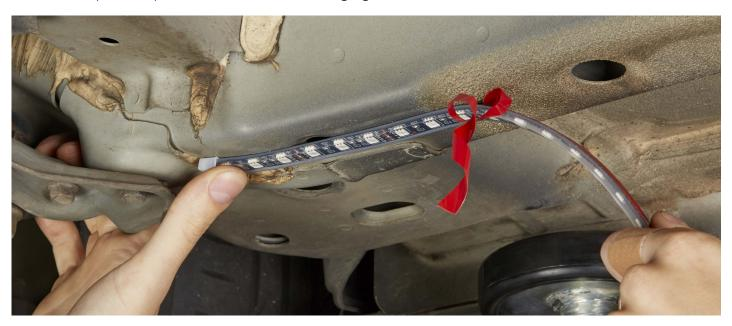
**STEP 5.** Route all light harnesses to a central location towards the front of the car, make sure they all reach the location you plan on mounting the Bluetooth controller. We recommend installing the controller inside the passenger compartment. If you are mounting the controller inside the vehicle, run the RGB wires through your firewall or floor. It is recommended to send the wires through one of the rubber grommets or floor plug.
