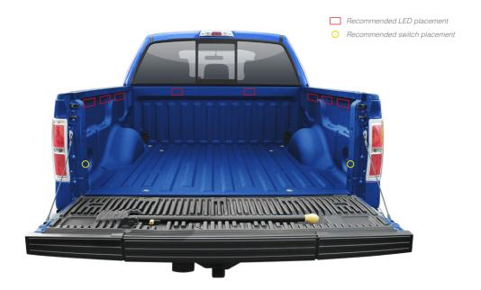
We recommend installing the lights within sheet metal recesses (if your pickup bed walls have them), again to minimize damage from any loose items.
