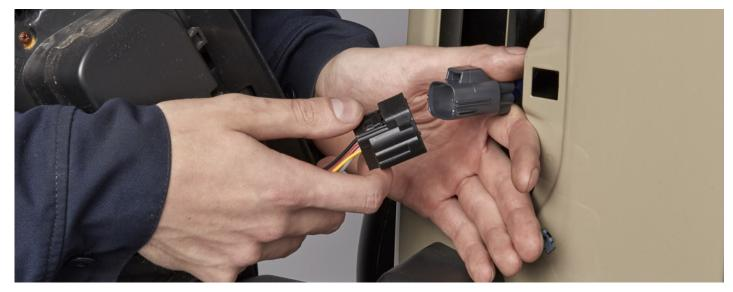
**STEP 6.** Place the vehicle in the "RUN" position (without starting the engine). Engage the parking brake and move the gear selector to the reverse position. Confirm the reverse lights are illuminated on the tail light you did not remove.
