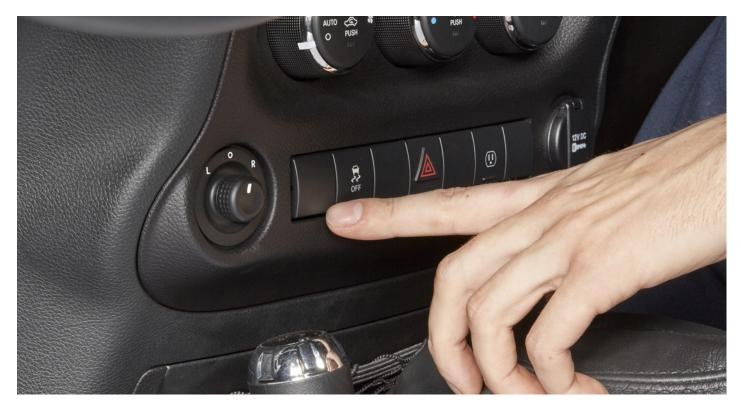
Once you find your mounting location, ensure there are no crucial components behind the area you will be installing the switch. Drill a <sup>3</sup>/<sub>4</sub>" hole, send the switch wires through the hole, plug in the switch, then snap the switch into the hole. An alternative option to using our switch is installing a switch panel, which is very helpful if you will be installing multiple accessories.
