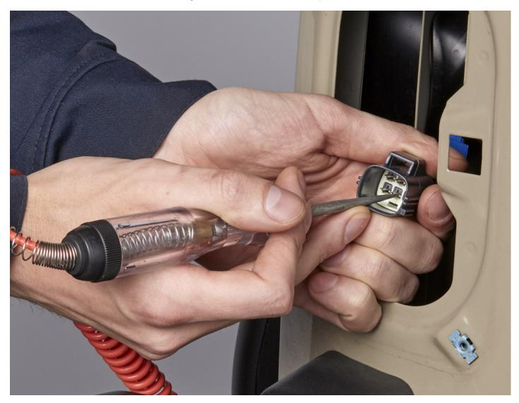
**STEP 8.** Find a suitable location to tap into the reverse light wire. Cut off the connector from the end of the light harness and separate the power and ground wire. Using a scotch lock or wiretap, connect the reverse light wire to the power (red) wire for the flush mount lights.
