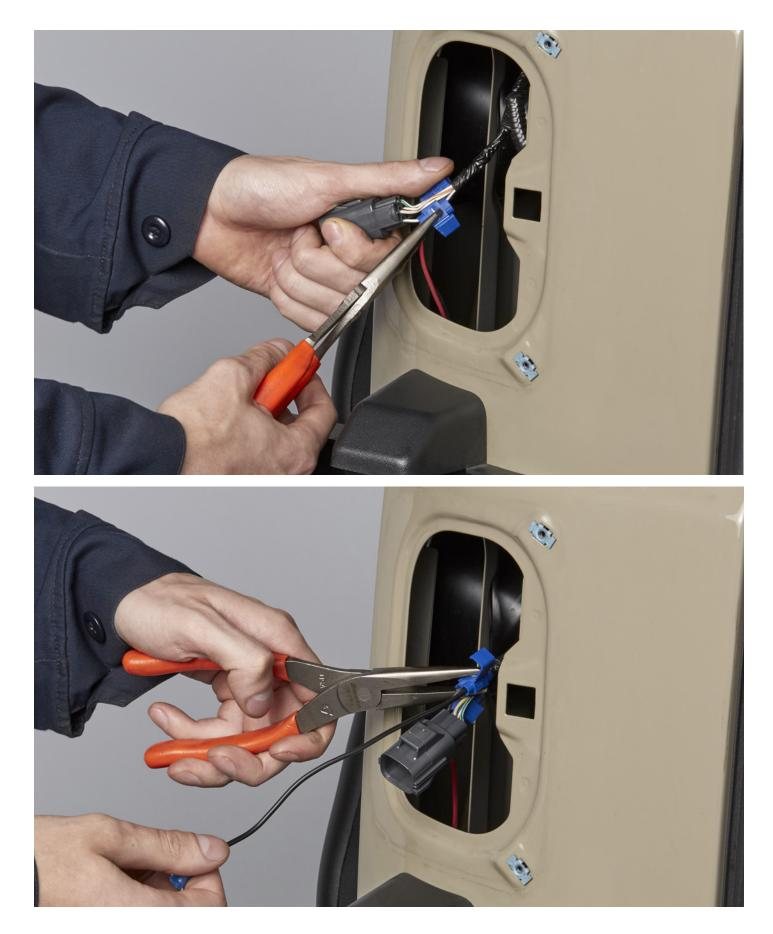
**STEP 9.** Connect the ground wire for the flush mount lights to a good ground on the body/frame, or you can connect it to the ground wire of the tail light harness using the same method described in step 6. You can locate the ground wire of the tail light by connecting the clamp of the test light onto the positive terminal of the battery and testing the terminals as described in step 5, the ground wire is usually black or white with a black tracer.
