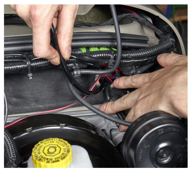
To ease installation, unplug the switch before you send the wires through the firewall. You can send the wire through an existing hole in the firewall, there is usually a rubber grommet in the hole of the firewall, make sure the grommet is still sealed when you are done running the wire.
