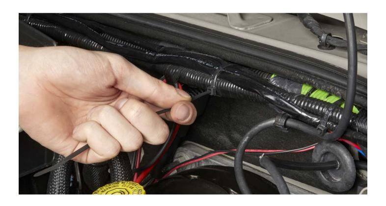
**STEP 5.** Run the wires for the switch through the firewall into the passenger compartment.
