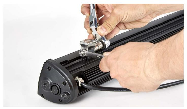
**STEP 8.** Make sure the light is properly installed and the mounts are secure.
