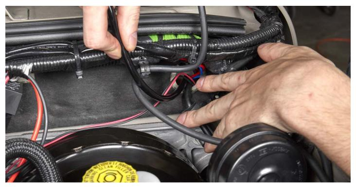
To ease installation, unplug the switch before you send the wires through the firewall. You can send the wire through an existing hole in the firewall, there is usually a rubber grommet in the hole of the firewall, make sure the grommet is still sealed when you are done running the wire.
