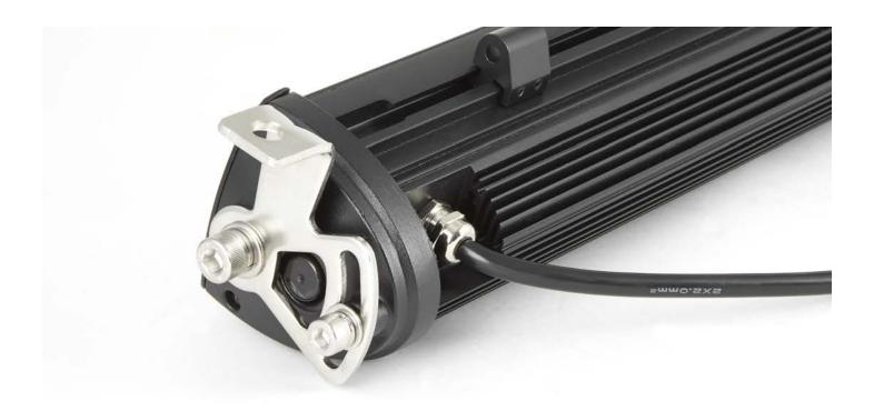
**STEP 2.** Install the pedestal mounts to the light bar using the provided hardware. The smaller bolt is installed to the rear of the light and allows for angle adjustment, the larger bolt is installed in the front and secures the light to the bracket.
