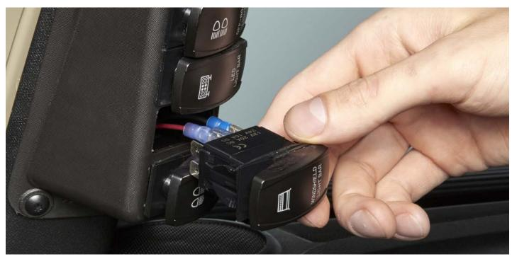
**STEP 7.** Now that you have the switch and light properly installed and connected, the final step is to connect the harness to the battery. Connect the ring terminal with the red wire to the positive terminal on the battery. Connect the ring terminal with the black wire to the negative terminal on the battery. Tuck away any remaining loose wires with cable ties.
