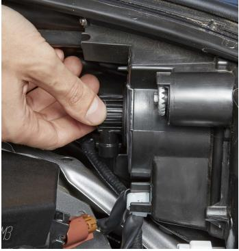
**STEP 5.** While looking into the headlamp from the front of the vehicle, ensure the bulb is in the correct orientation according to the adjustment instructions included in the box.
