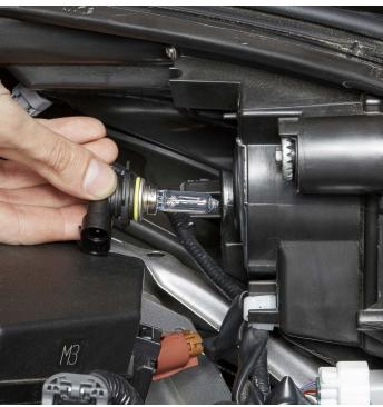
**STEP 4.** Place the new G10 LED conversion bulb in the socket and make sure it is secure.
