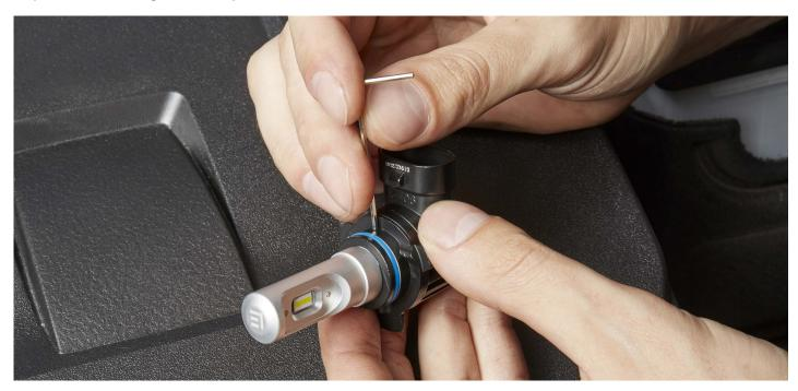
**STEP 7.** Once the bulb is properly situated, plug the bulb into the headlight harness. Do not re install OEM dust covers, to allow for adequate cooling of conversion bulbs.
